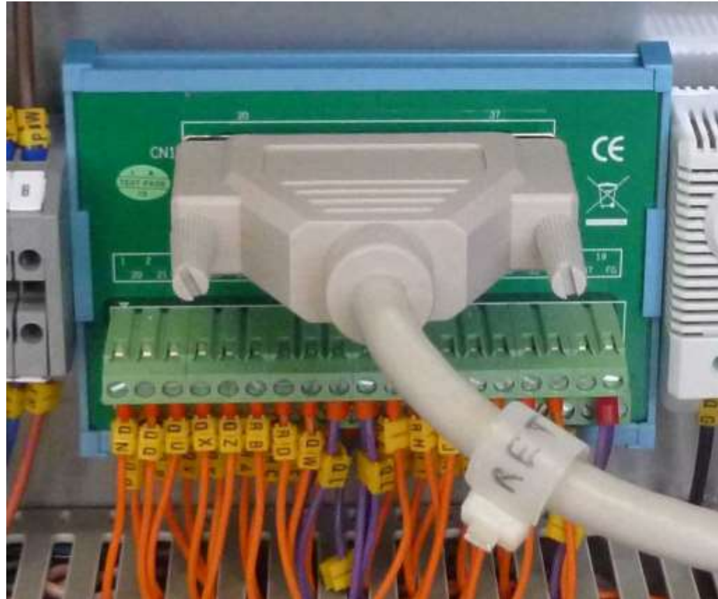
Interface connectique ADVANTECH ADAM 3937.
